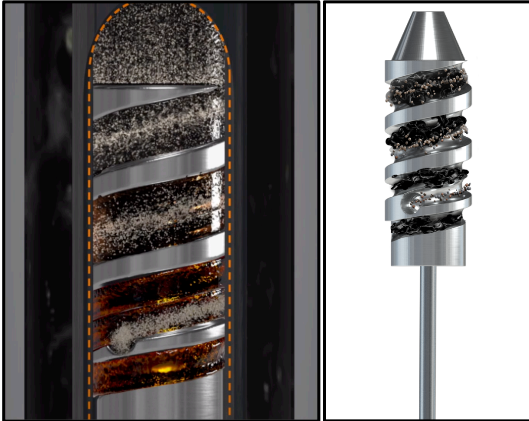
Figure 6: Structure of the dual-channel spiral.
