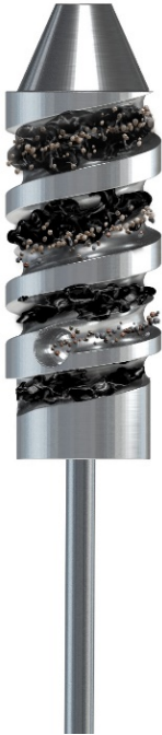
FIGURE 4: Illustrates an in-depth look at the sand separator portion of the Super Max. As shown, the dual-channel spiral encourages heavier sand particles to fall into the lower channel, while lighter fluids are retained in the higher channel. Solids are then funneled into the sand drain and eventually fall into the sand bypass tube, where they are then deposited into the mud joints. Fluid exits the bottom of the centrifuge and enters the pump suction.
