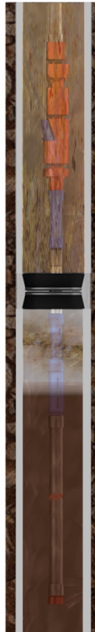
FIGURE 1: Picture of gas overtaking ESP pump.
